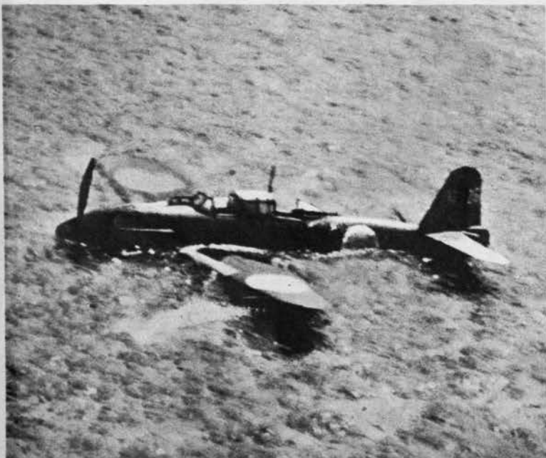
Long nose containing an inline engine helps identify Judy, carrier-based recco plane and divebomber. Water hides the prominent radiator below engine but helps bring out the position of Judy's midwing.
